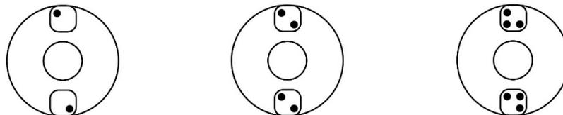
*Buckets can be placed around the rotor in any of the rotor loading configurations shown.
